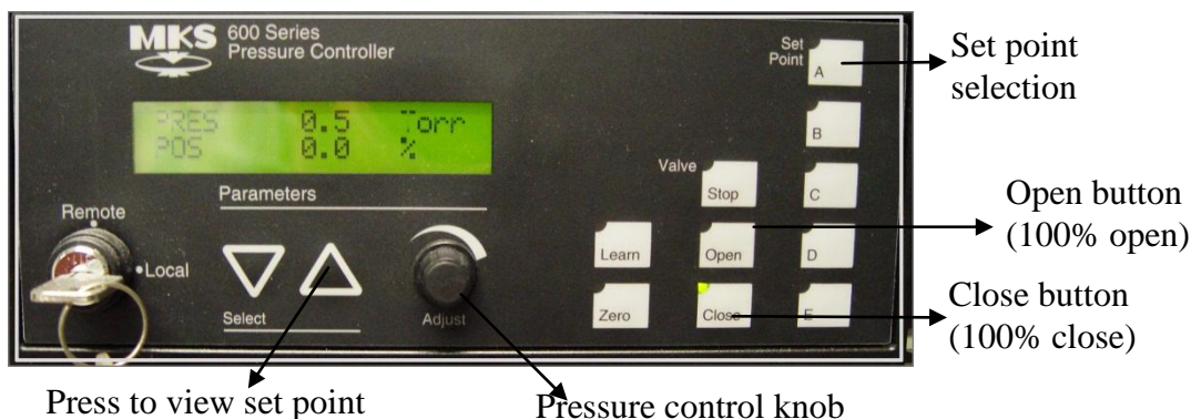
Figure E.8: pressure controller front panel.
